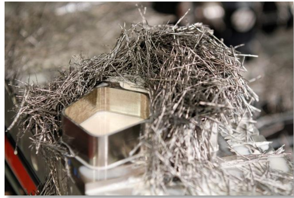
Before and After - Machining Titanium at 5 cu. in per min with ½” tool at 1” in depth
